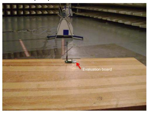
Set-up for Spurious Emissions 1GHz – 12.75GHz
