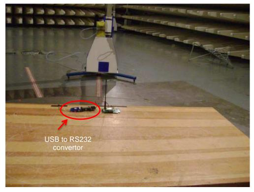
**Set-up for Conducted Emissions**
