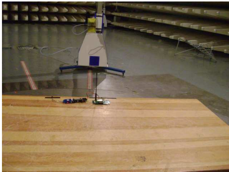
Photograph 2: Set-up for Spurious Emissions 1GHz – 12.75GHz
