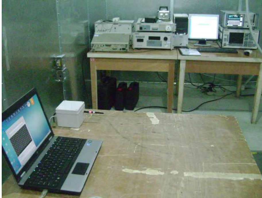
Photograph 3: Set-up for Conducted Emissions
