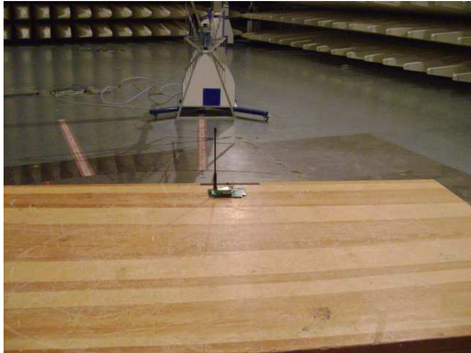
Photograph 1: Set-up for Spurious Emissions 30MHz – 1GHz
