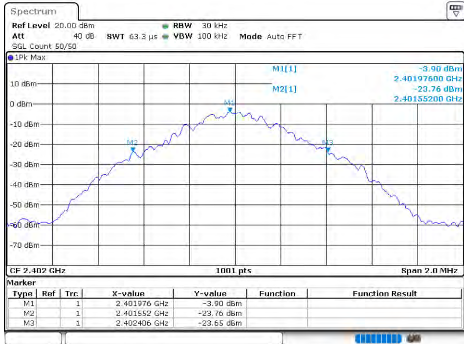
-20 dB BW NVNT 1-DH5 2402MHz Ant1
