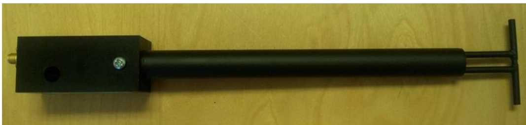
Figure 1 – MVG COMOSAR Validation Dipole
