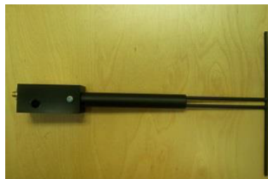
Figure 1 – MVG COMOSAR Validation Dipole
