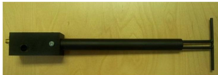
Figure 1 – MVG COMOSAR Validation Dipole
