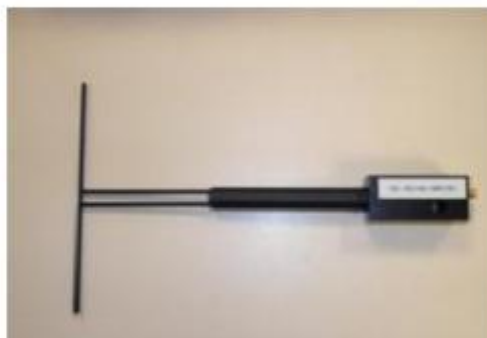
Figure 1 – Satimo COMOSAR Validation Dipole
