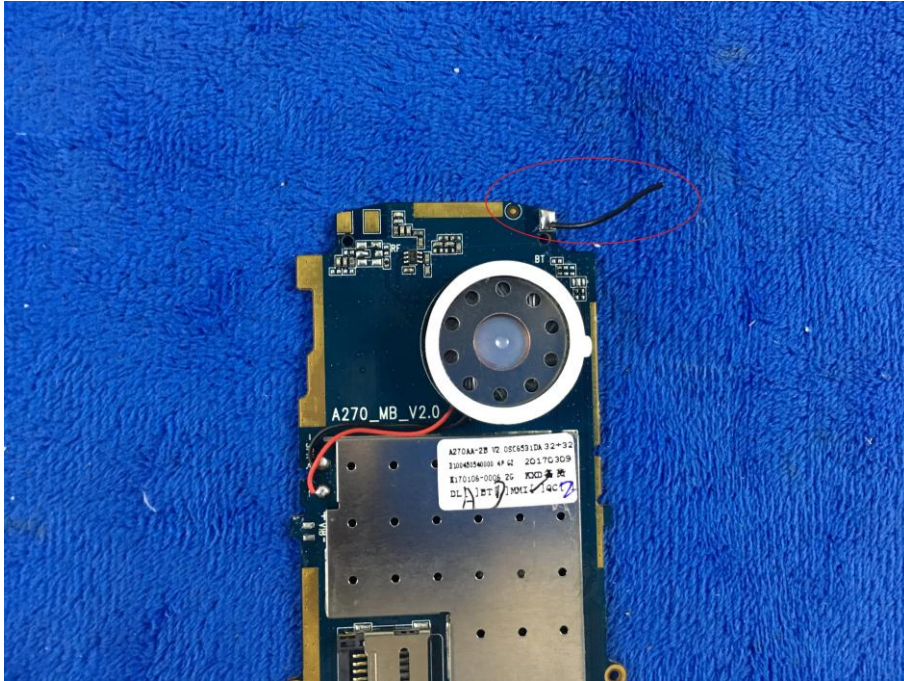
BT - Antenna View
