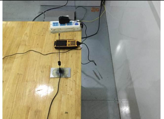
Conducted Emissions Test Setup Side View
