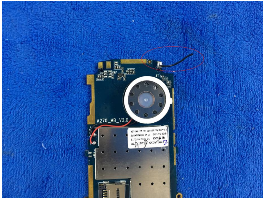
BT - Antenna View
