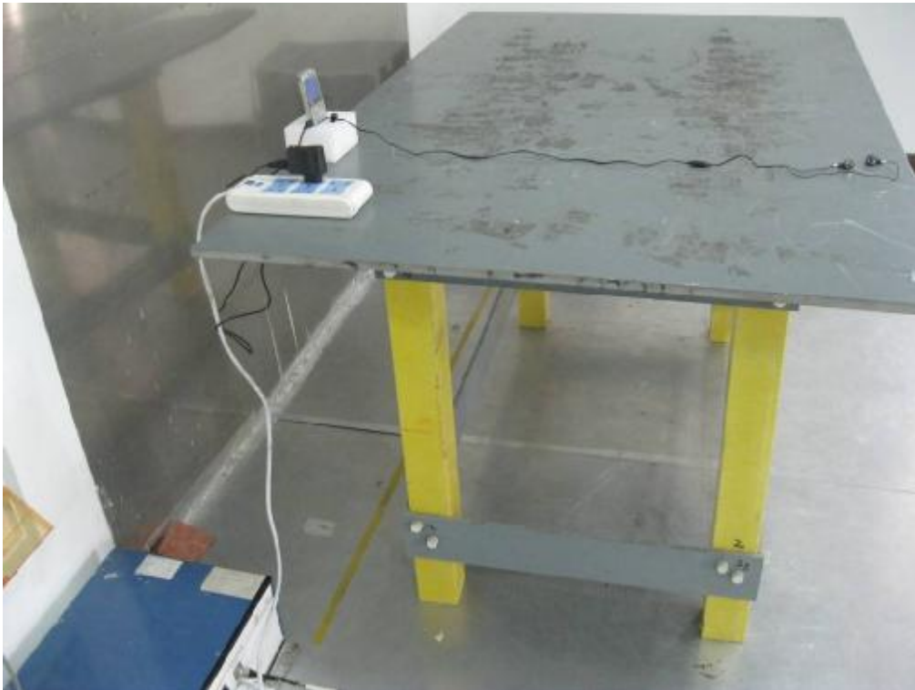
Conducted Emissions Test Setup Side View
