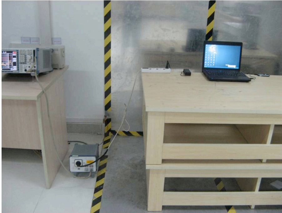
FCC LINE CONDUCTED EMISSION TEST SETUP
