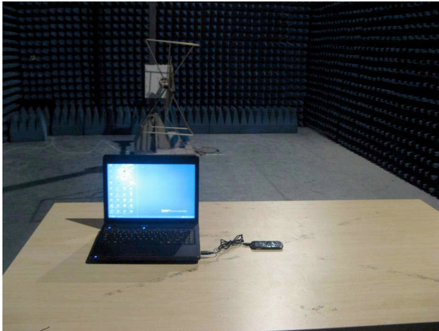
FCC RADIATED EMISSION TEST SETUP
