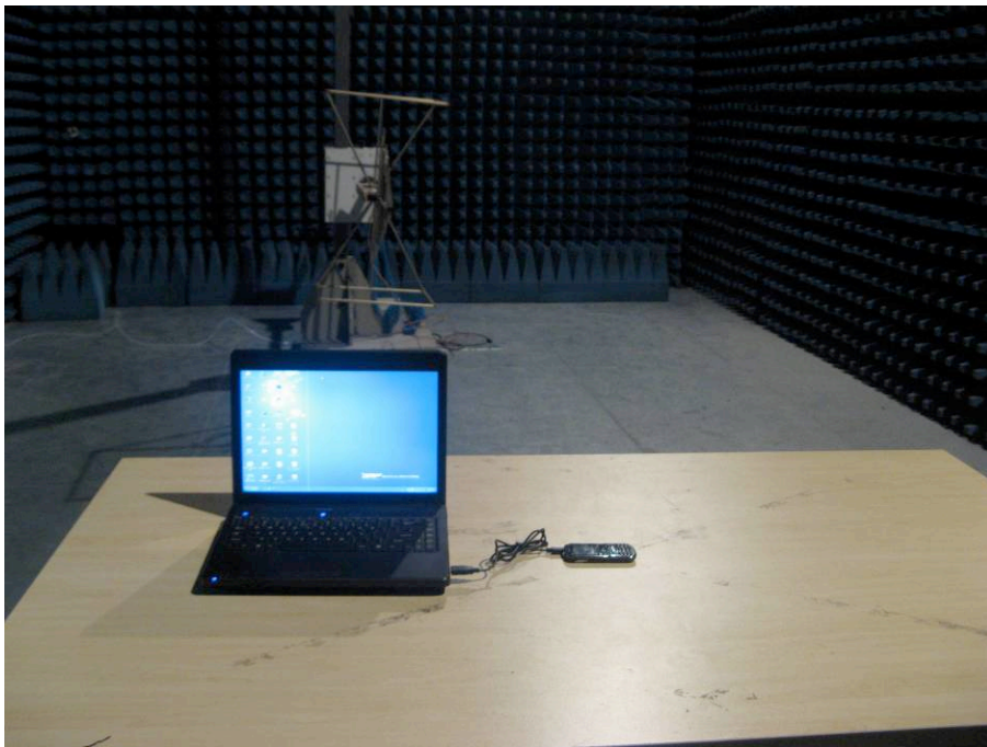
FCC RADIATED EMISSION TEST SETUP
