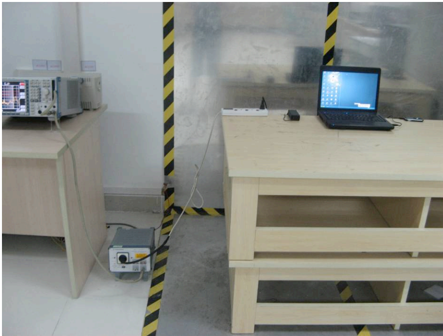
FCC LINE CONDUCTED EMISSION TEST SETUP
