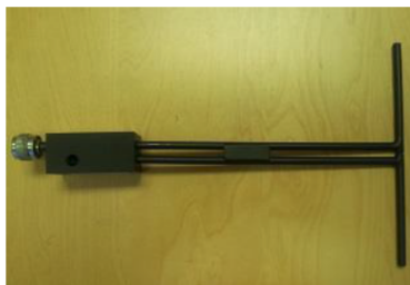
Figure 1 – MVG COMOSAR Validation Dipole
