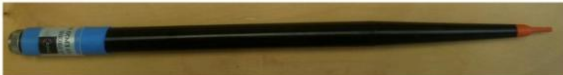
Figure 1 – MVG COMOSAR Dosimetric E field Dipole
