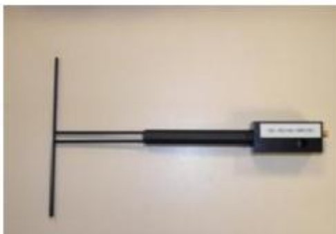
Figure 1 – Satimo COMOSAR Validation Dipole
