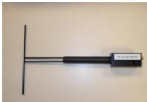
Figure 1 – Satimo COMOSAR Validation Dipole
