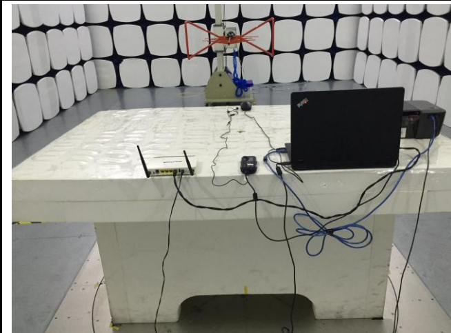
Radiated Emissions Test Setup Below 1GHz
