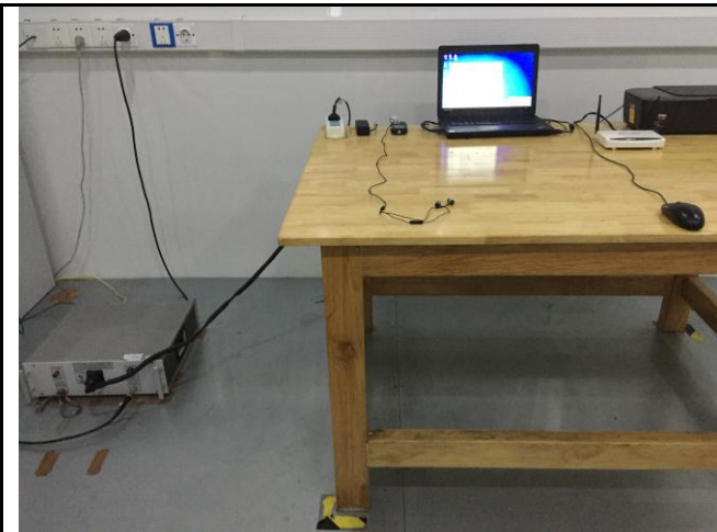
Conducted Emissions Test Setup – Front View
