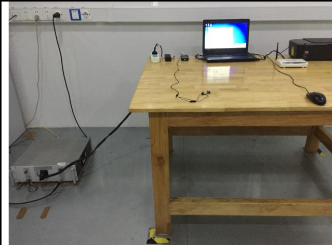
Conducted Emissions Test Setup – Front View
