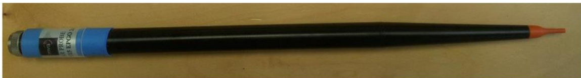
Figure 1 – MVG COMOSAR Dosimetric E field Dipole
