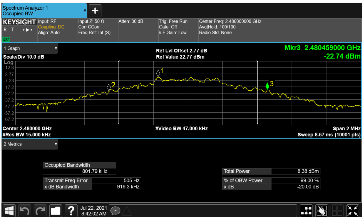
-20dB Bandwidth NVNT 2-DH1 2402MHz Ant1
