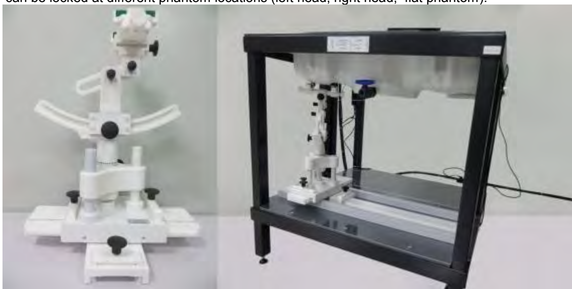
Device holder supplied by SATIMO
