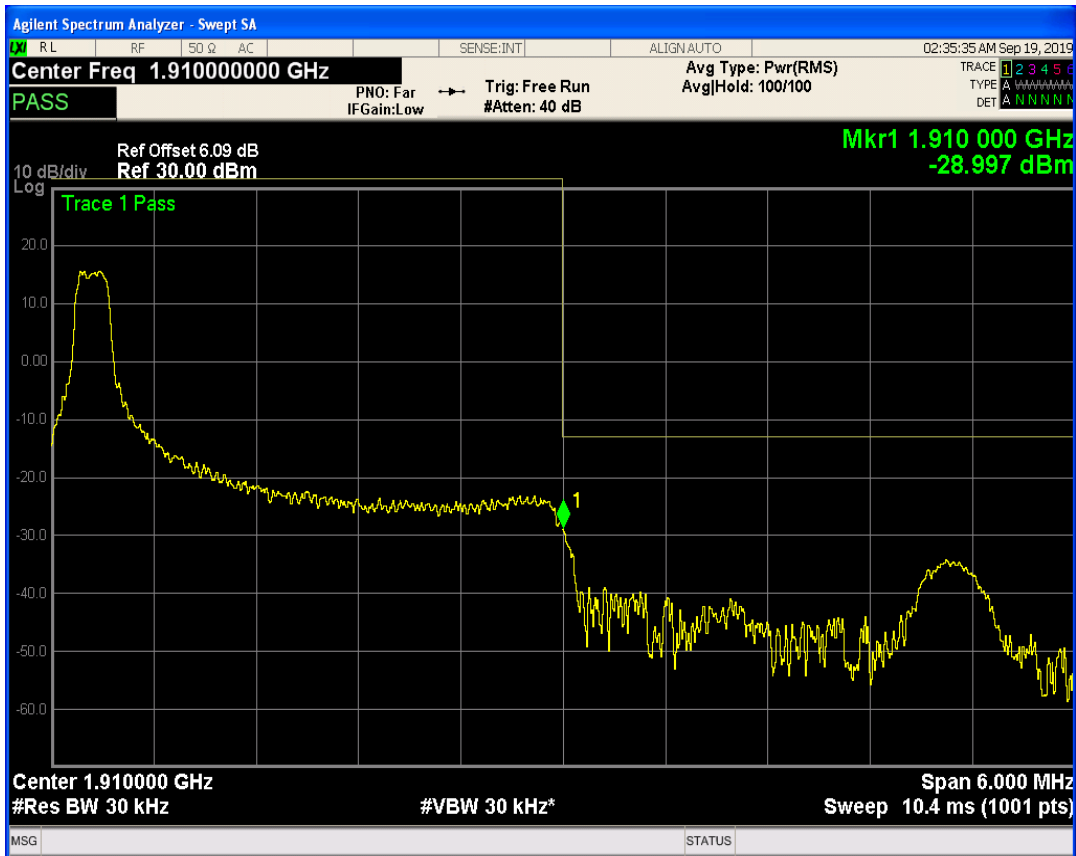
LTE Band2 QAM16 BW=3MHz Channel=19185 RB Size=1 Position=#0
