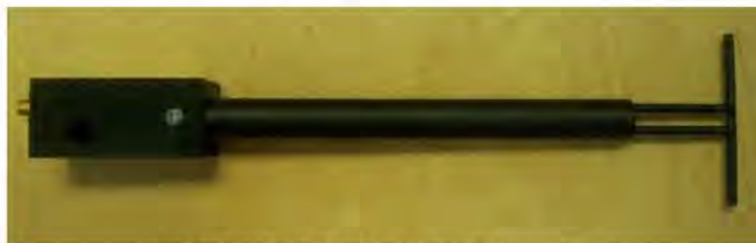
Figure 1 – MVG COMOSAR Validation Dipole
