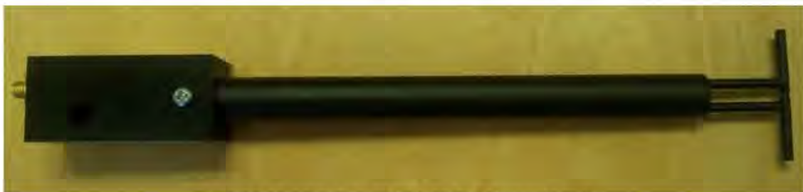
Figure 1 – MVG COMOSAR Validation Dipole
