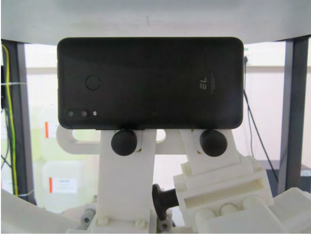
10mm body-worn Left Side Setup Photo(hotspot)
