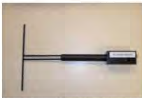
Figure 1 – Satimo COMOSAR Validation Dipole
