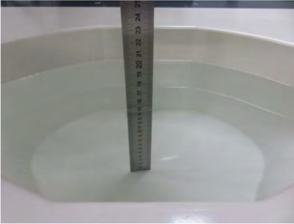
Photograph of the depth in the Body Phantom (2450MHz, 15.2cm depth)
