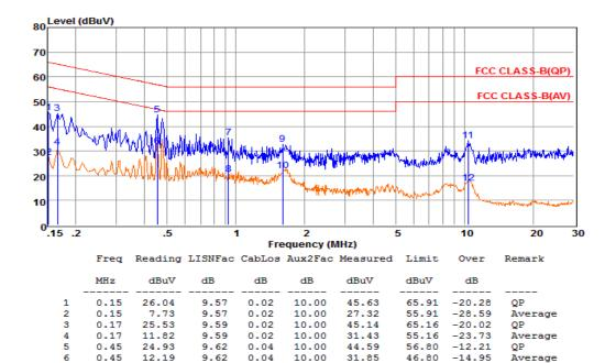
Remarks: 1. Measured = Reading + LISNFac + Cable Loss + Aux2 Fac.
