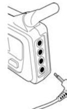
If you decide to use the handle bar mount PTT button, place the wired PTT button on the left side handle bar grip (closest to where your thumb would be) of the motorcycle using the integrated Velcro strip. And insert the 2.5mm plug into the PTT input in the back of the main unit.
