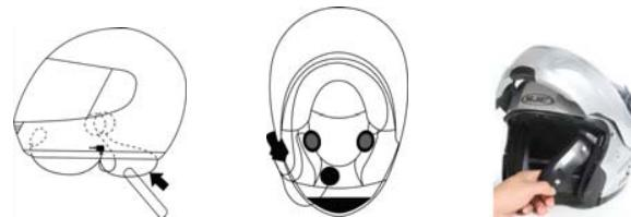
Fasten the mounting bracket snugly to the bottom left side of the helmet with two bolts supplied. Align the back side of the X1 slim unit to the grooves on the mounting bracket. Slide the X1 slim unit down on the mounting bracket until it latches firmly into place.
