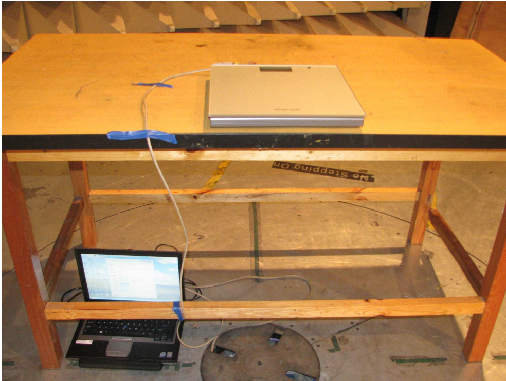
Photograph 2: Radiated emission orientation of the sample on the table
