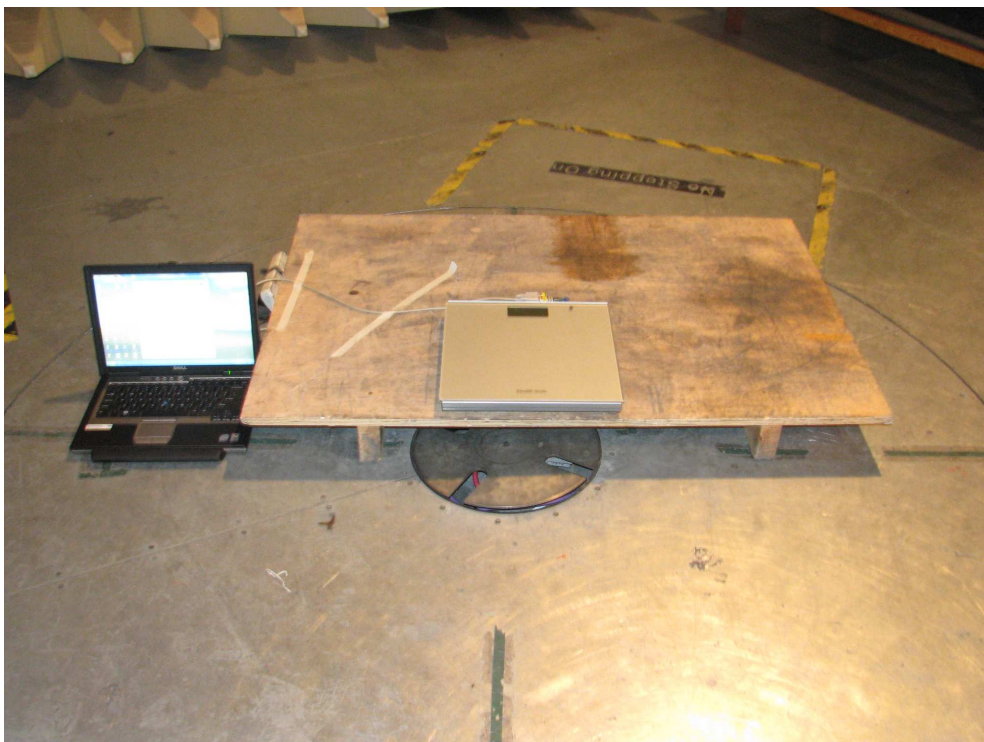
Photograph 3: Radiated emission orientation of the sample on the wood support
