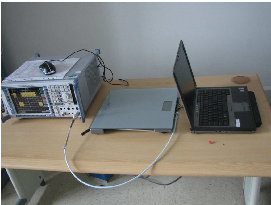
Photograph 1: Set-up for Conducted Emissions at Antenna Port
