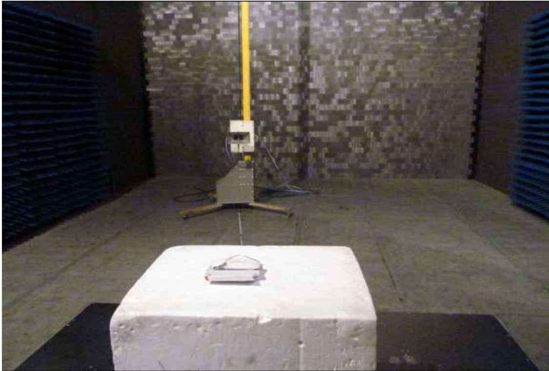
Photograph 4: Set-up for Radiated Emission, 1G-18GHz
