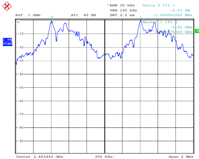
Figure 1: Carrier Frequency Separation-Low Channel
