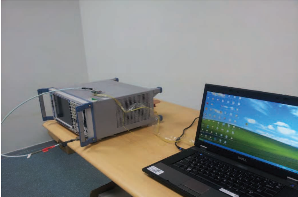
Photograph 1: Set-up for Conducted Power at Antenna Port
