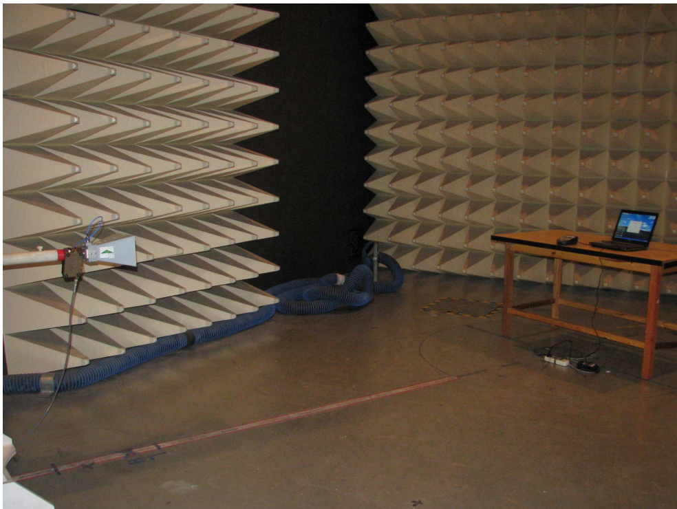
Photograph 4: Set-up for Radiated Emission, 1G-18GHz
