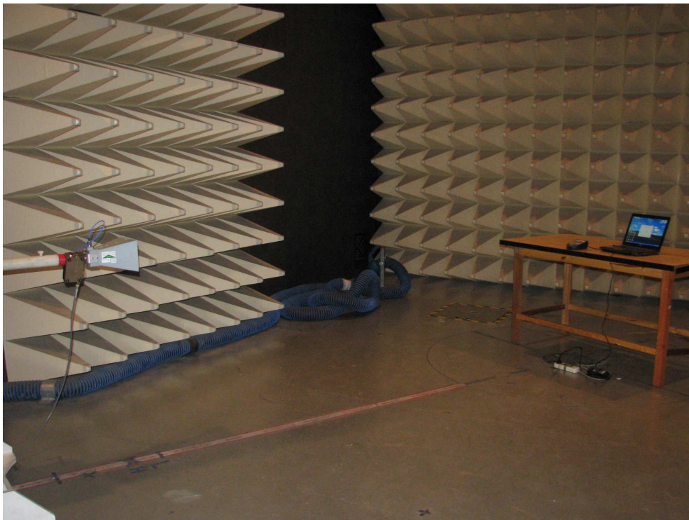
Photograph 4: Set-up for Radiated Emission, 1G-18GHz
