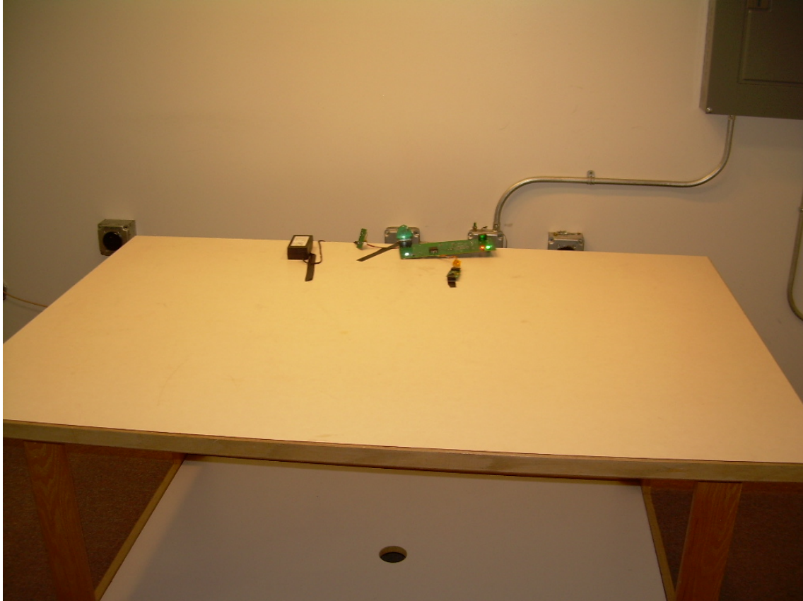
Photograph 3 – Front View Conducted Disturbance Worst Case Configuration
