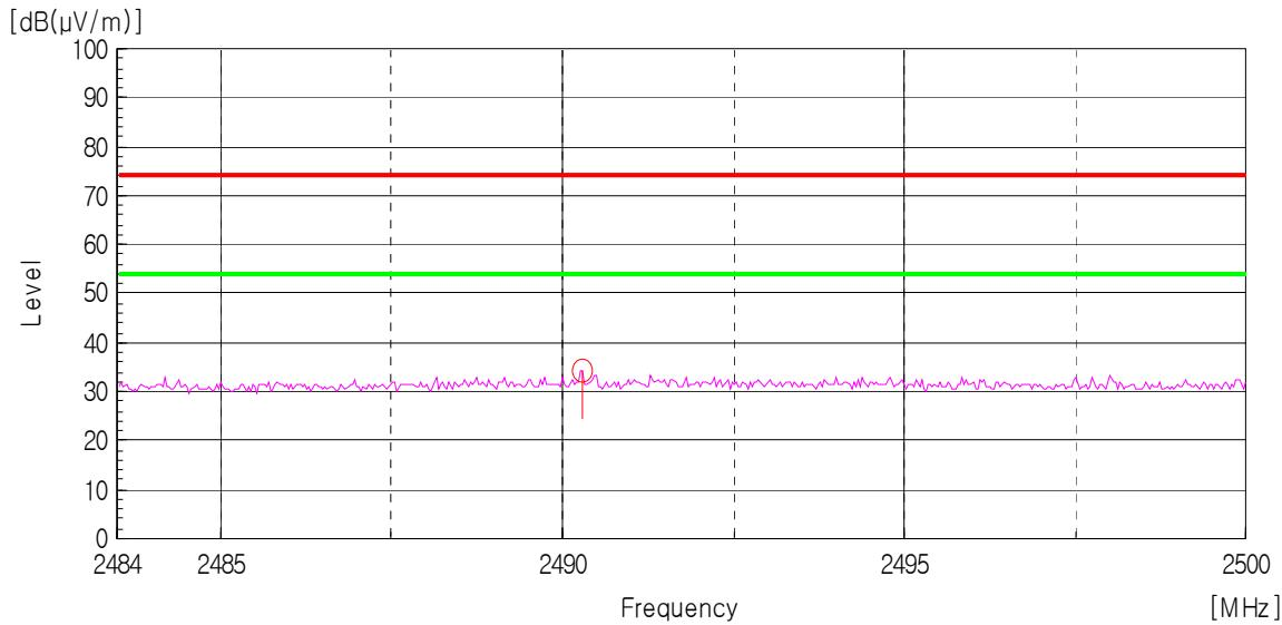
AV Detector: RBW: 1MHz, VBW: 10 Hz (2 483.5 MHz - 2 500.0 MHz), Worst case (High, Vertical)
