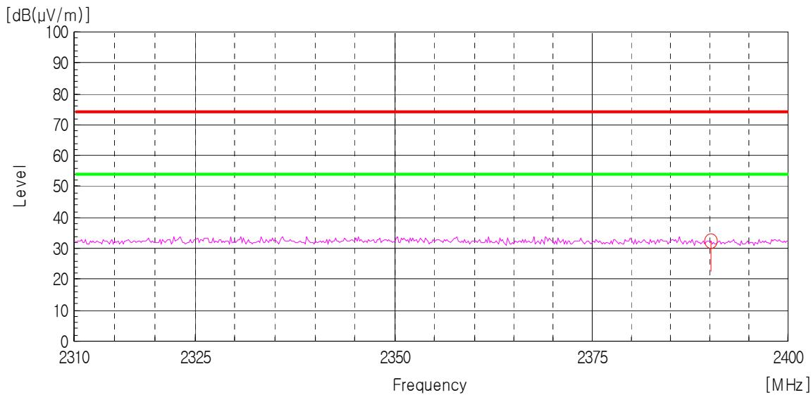
AV Detector: RBW: 1 MHz, VBW: 10 Hz (2 310 MHz - 2 410 MHz), Worst case (Low, Vertical)
