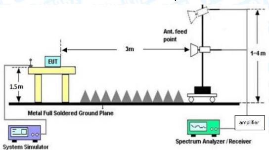
**Above 1GHz Test Setup**
