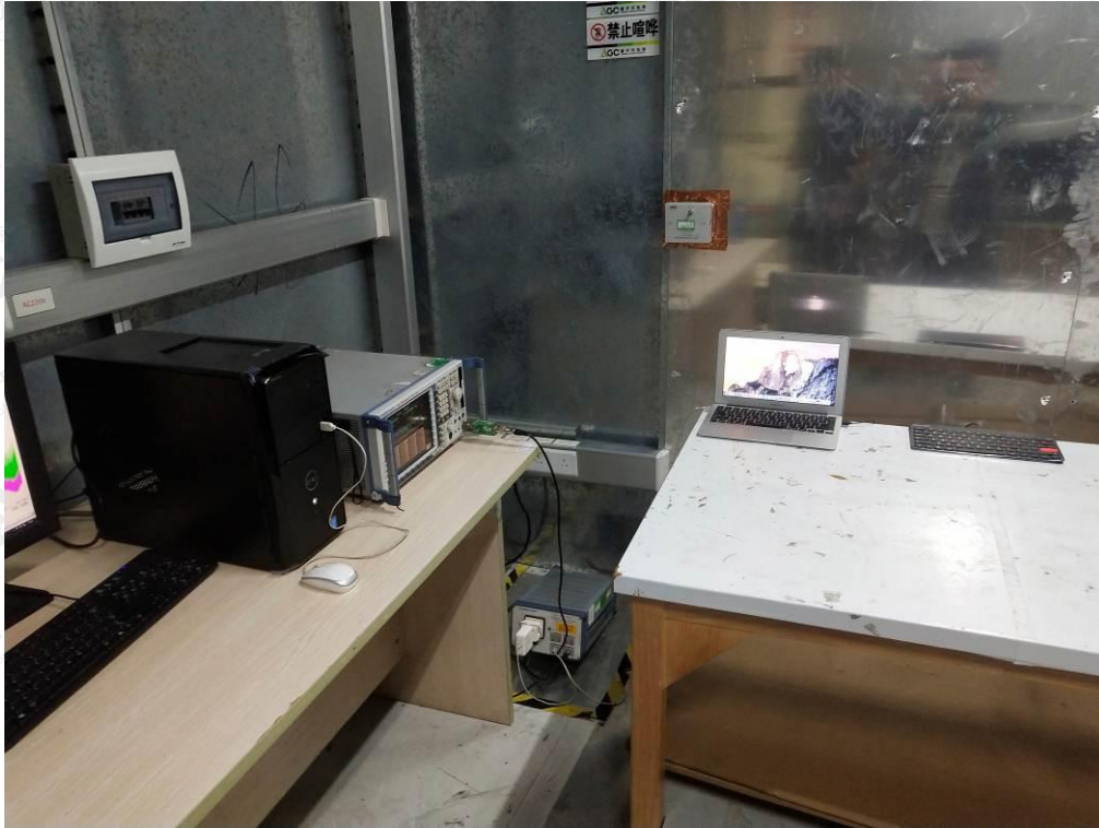
FCC RADIATED EMISSION TEST SETUP
