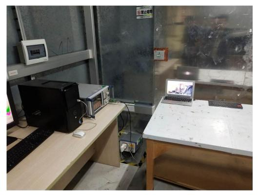
FCC RADIATED EMISSION TEST SETUP
