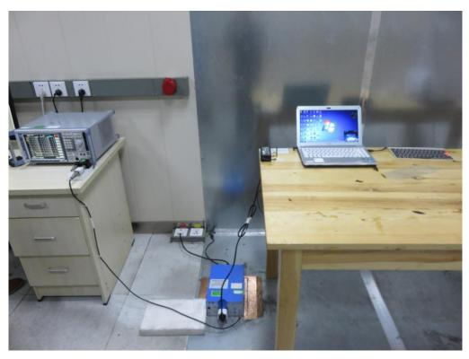
FCC RADIATED EMISSION TEST SETUP
