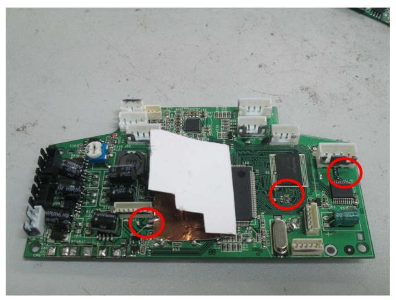
5.The R9, R10 changed to 0 ohm. in U5 ,the 21,23 pin each add a 600 ohm @100M bead and 10PF capacitors to GND; in J2, J3 of 29 pin add a 104PF capacitor, J1, J2 connected PCB board of 1pin and 15-23 pins add a 100.@100M bead $_{\circ}$
