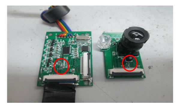
6.In U8 of the 6 pin add a 600 ohm @100M bead and add 10PF capacitors to GND; in J11 of the 4-7 pins add a 100 @100M bead and add a 33PF capacitor to GND $_{\circ}$
