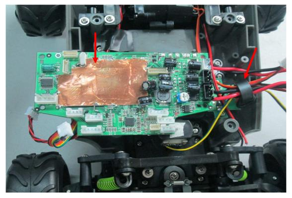
2.Two row line need shielding and grounding; In J5, J6 ports of cable add a core and around 2 times, core model: ; In J24, J20 ports of cable add a core and around 2 times, core model: T18\*6\*10; in J13, J22, J4 ports of cable add a core and around 2 times, core model: T18\*6\*10; In J11 port of cable add a core and around 3 times, core model: T18\*6\*10; add a shielding on the PCB.
