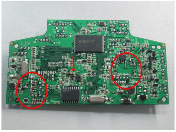
4.Connect R21 ends of signal line each add a 33 ohm resistor, in J11 , J20 of D+ D-, add a 60 ohm @100M bead  $_{\circ}$
