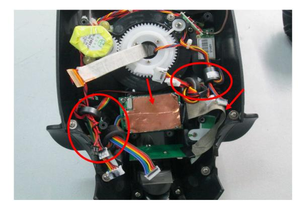
3.In C60, C11, C118, add a bead of 300 ohm @100M; in C54, C64, C119, C1118 add 104PF capacitor; in J5, D6 ports add 102PF of capacitor to GND; in J11 port add 10PF of capacitor to GND $_{\circ}$
