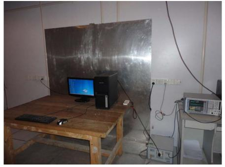
RADIATED EMISSION TEST BELOW 1GHz (For Transmitting)
