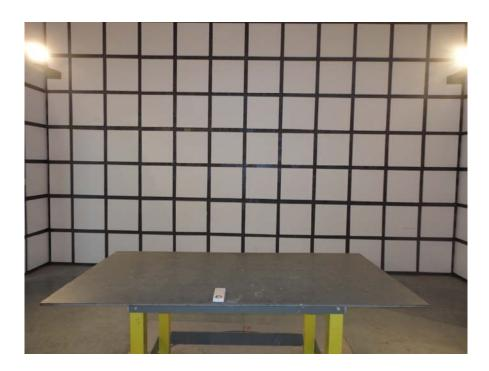
RADIATED EMISSION TEST ABOVE 1GHz (For Transmitting)
