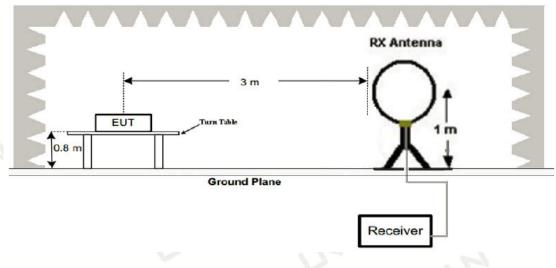
2. Radiated Emission Test-Up Frequency 30MHz~1GHz
