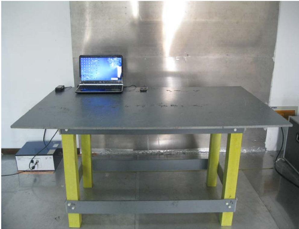
Conducted Emissions Test Setup - Front View
