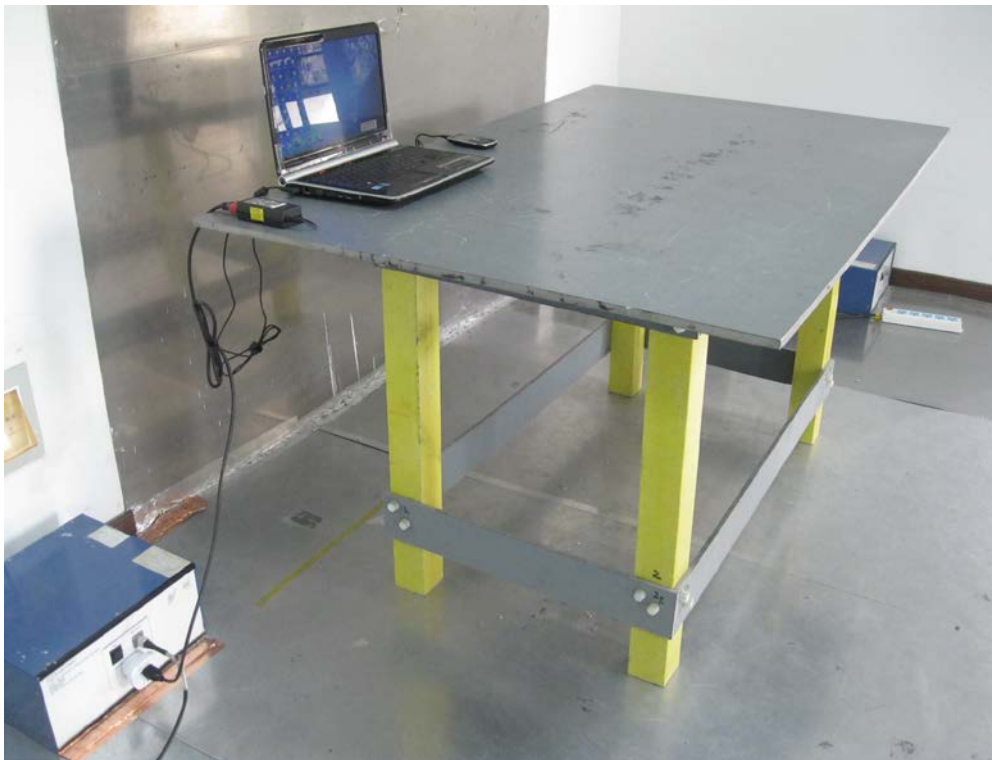
Conducted Emissions Test Setup - Side View
