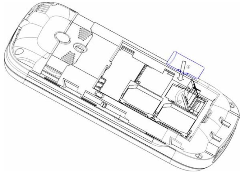
**Tip:** If you have some problem with the T-flash card, please check whether the T- flash card is installed properly or not and whether there is a good connection between the T-card and the socket or not.
