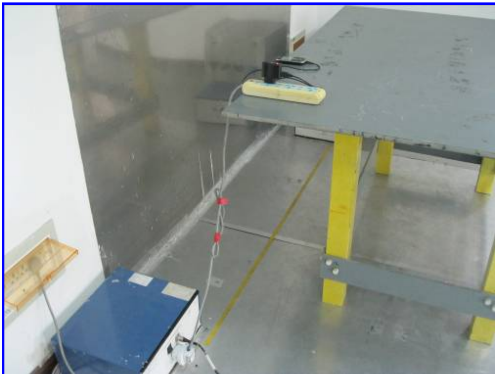
Side View of Conducted Emission Test Setup
