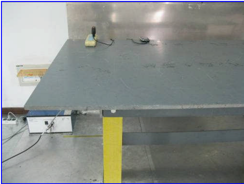
Front View of Conducted Emission Test Setup
