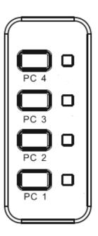
Buttons on panel are selection buttons. Just press one button and then you can select the corresponding port. Each button has upper and lower two LEDs indicating on line and selected status. The upper indicates the on line status. It lights if the corresponding computer is on line. The lower indicates the selected status. Since there is only one port selected at one time, the only one LED lights to show that the corresponding computer is selected.
