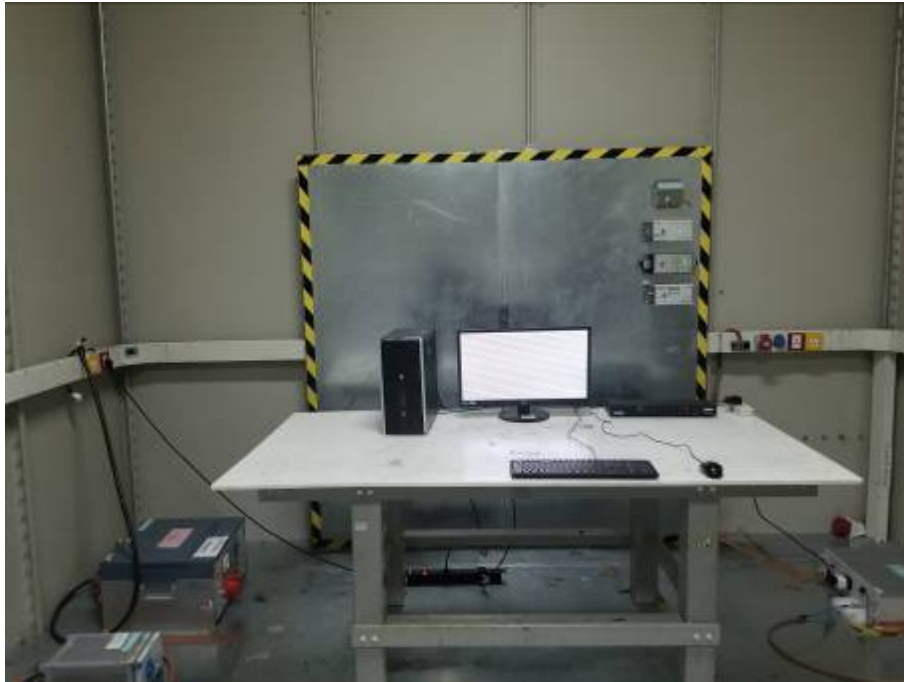
Front View of Conducted Emission Test
