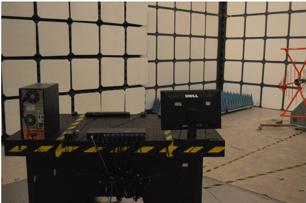
Back View of Radiated Emission Test (30MHz ~ 1GHz)
