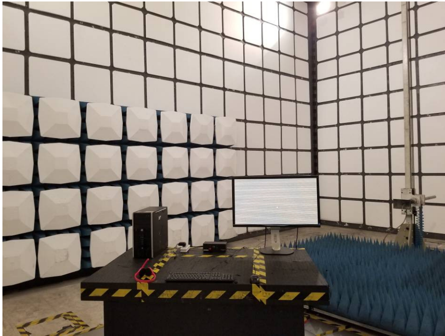
Front View of Radiated Emission Test (1GHz ~ 18GHz)
