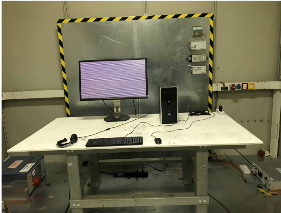
Front View of Conducted Emission Test
