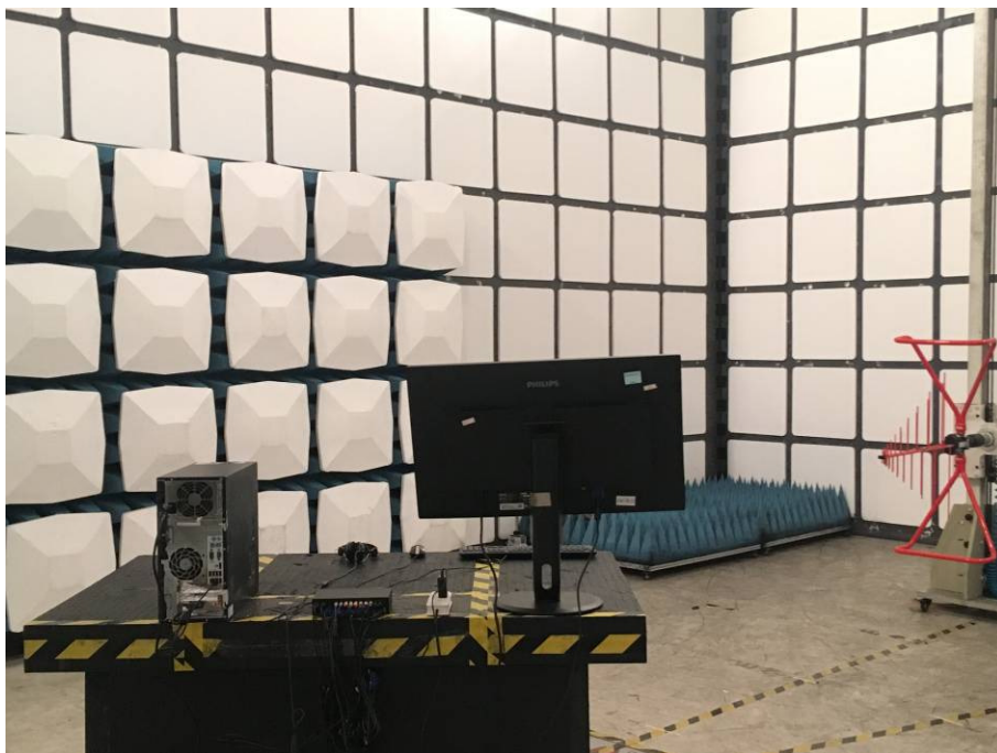
Back View of Radiated Emission Test (30MHz ~ 1GHz)
