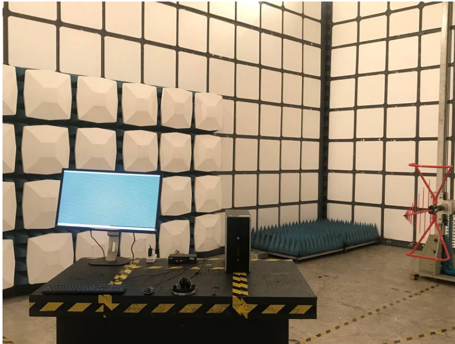
Front View of Radiated Emission Test (30MHz ~ 1GHz)
