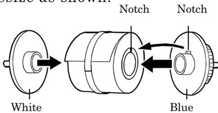
Install spacers in the paper flanges first when using L size paper or 5×7 size paper. When using 4×6 size paper or 6×8 size paper, proceed with Step 3 without installing the spacers.
