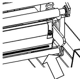
3. Using gauze dipped with isopropyl alcohol or ethyl alcohol, clean the rubber section of the platen roller
