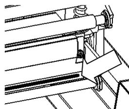
2. Using gauze dipped with isopropyl alcohol or ethyl alcohol, clean the edge of the peeling roller.
