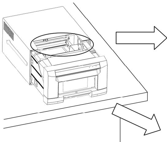
1. Using gauze, clean the heat element (glass bar) of the thermal head with isopropyl alcohol or ethyl alcohol.
