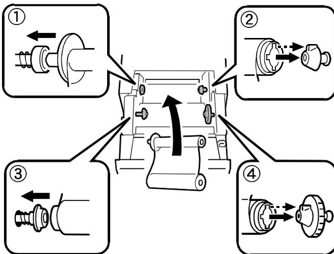
4. Take the slack the ink ribbon by turning the ink ribbon supply core.
