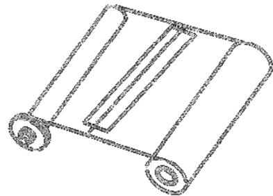
3. Turn the ribbon on the rewinding side and rewind the taped section completely.
