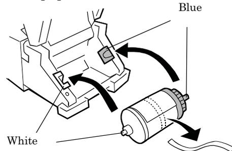
4. Insert the edge of paper under the guide roller by rotating the paper flanges. Insert the paper until the Paper Setting Lamp is lit.
