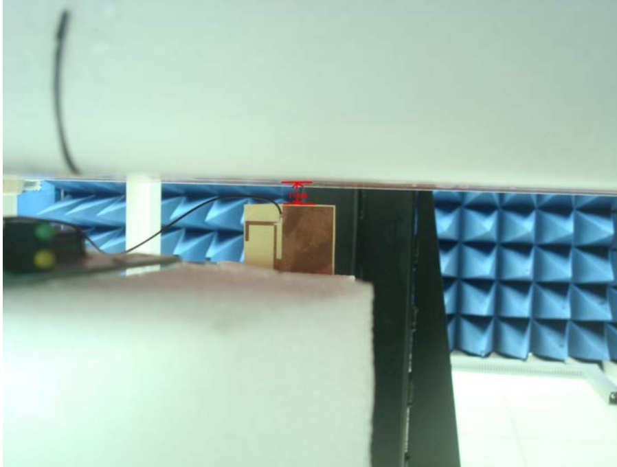
Figure 5. Body SAR Test Setup (Flat Section) _ Side E
