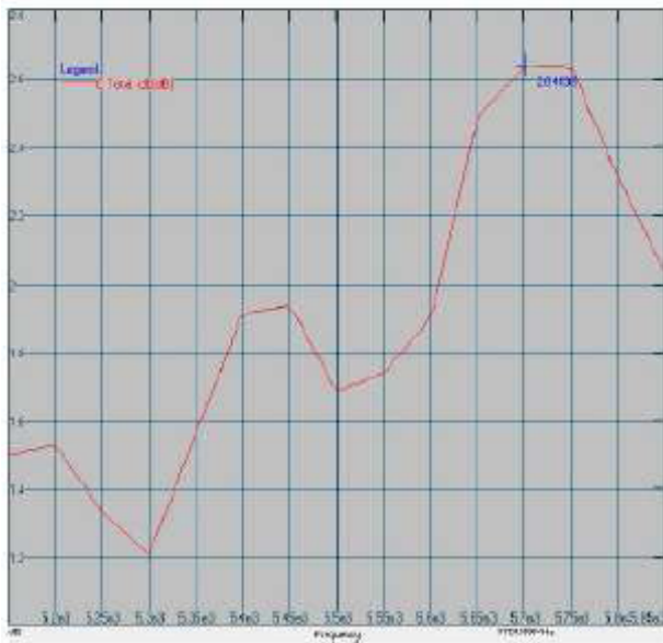
Maximum Peak Gain at 5701 MHz : 2.64 dBi
